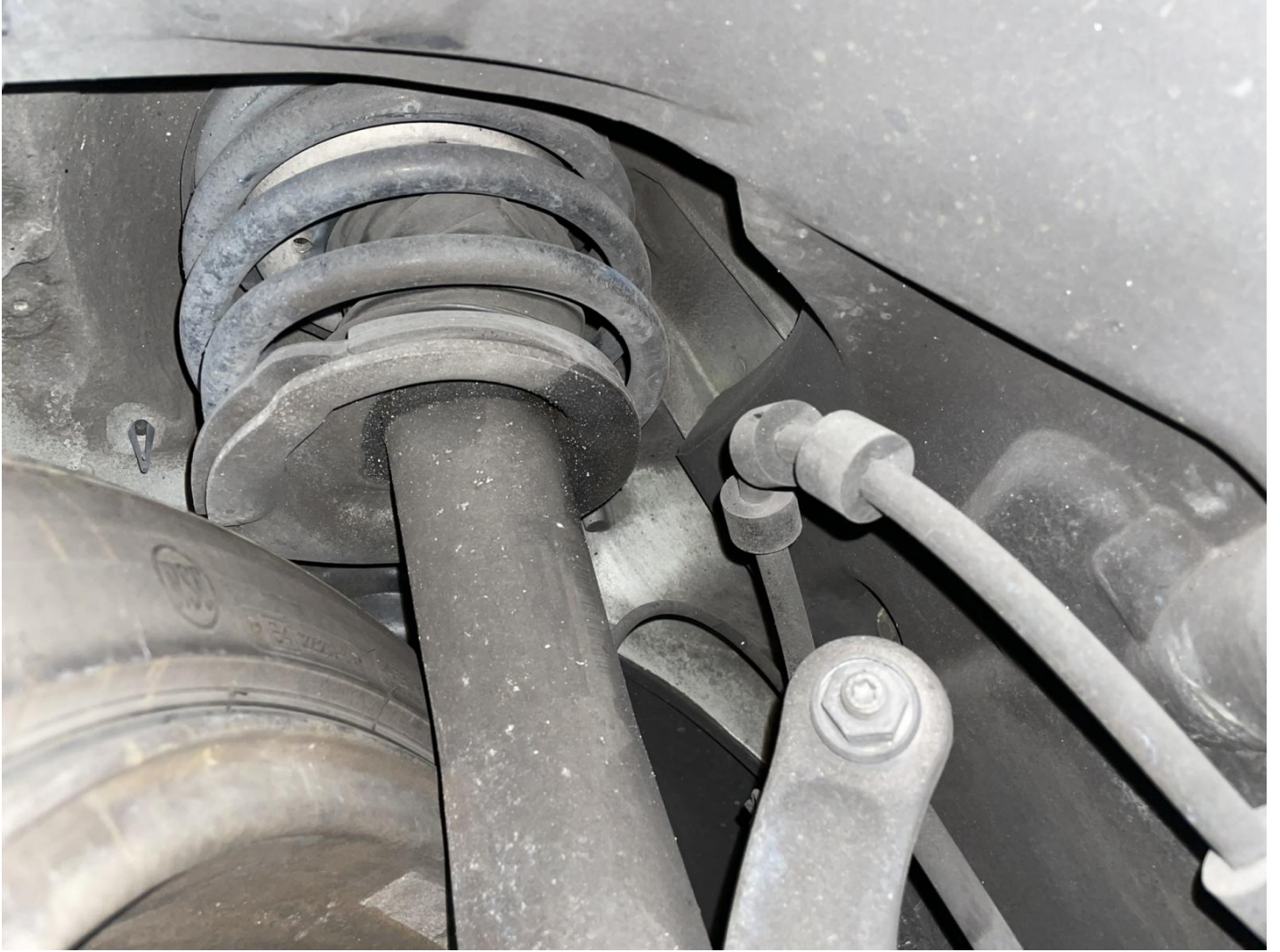
shock absorber oil leak
