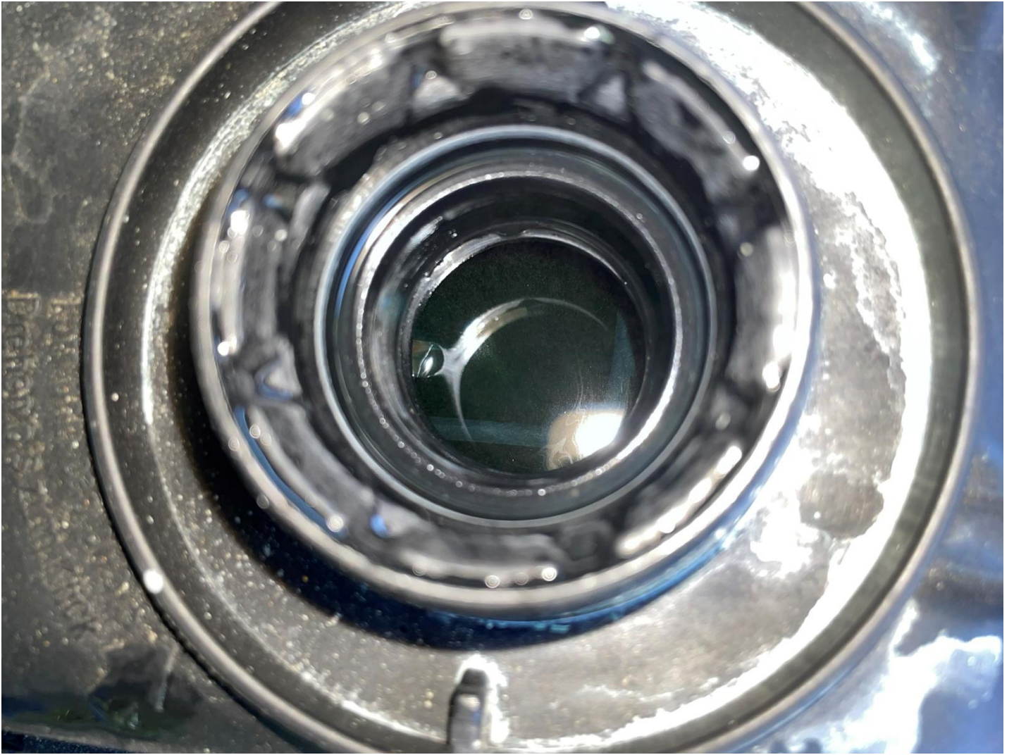
broken coolant level indicator
