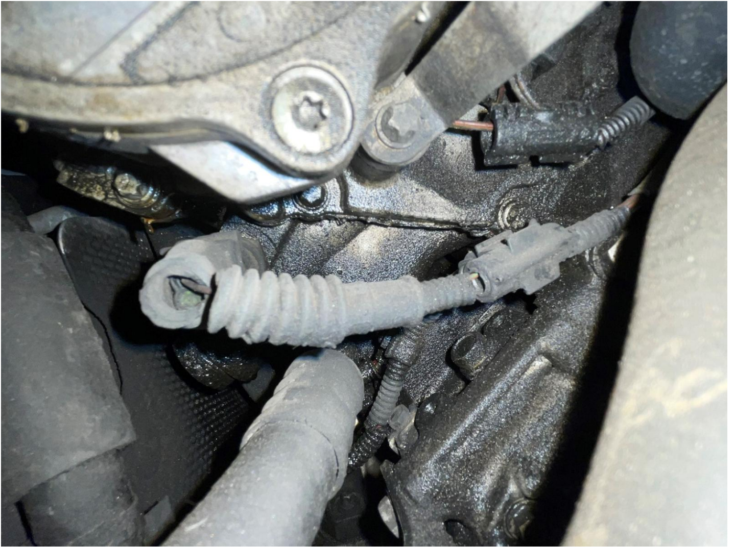
timing chain cover oil leak
