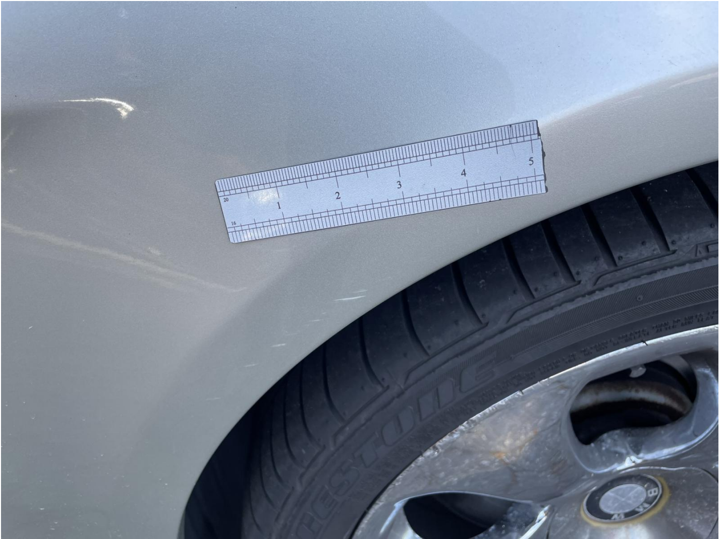
Body damage: Front left door
