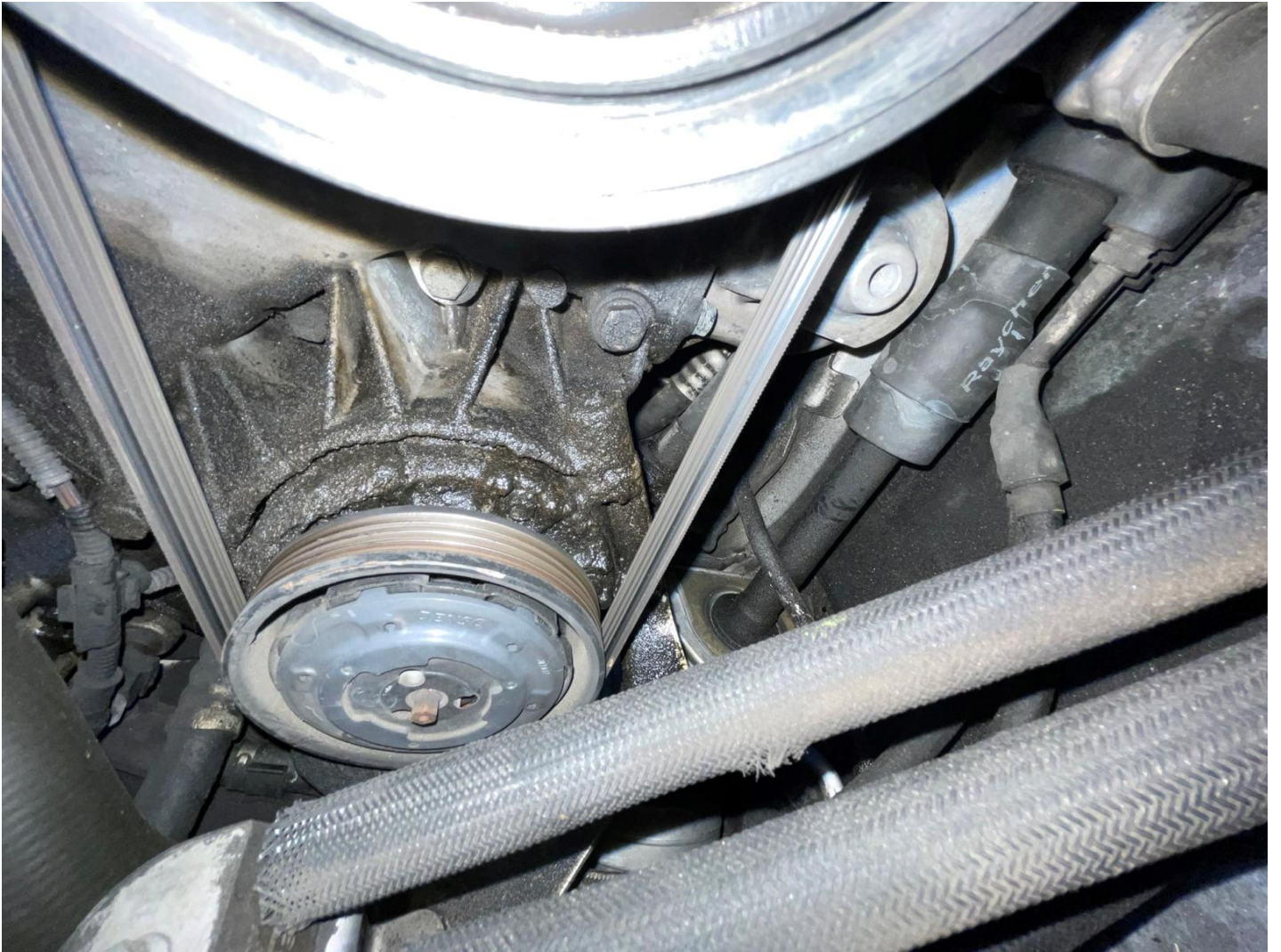
timing chain cover oil leak
