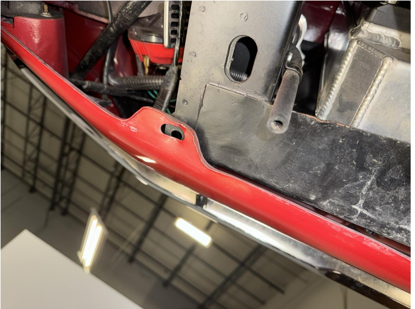
Body damage: Rear bumper
