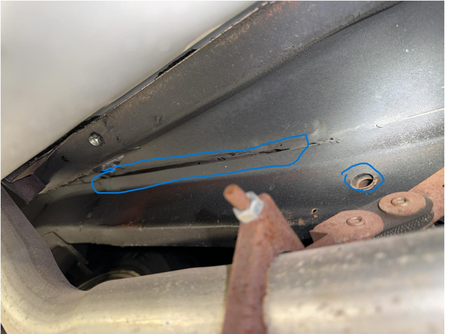
missing welding spots
