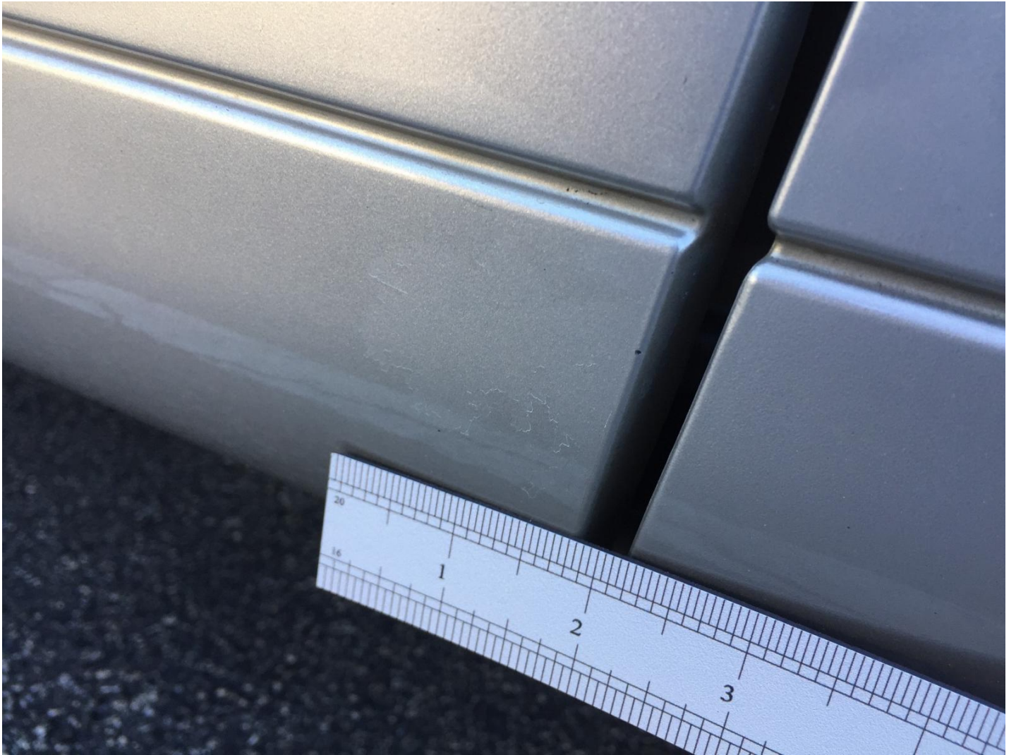
Clear coat peeling
